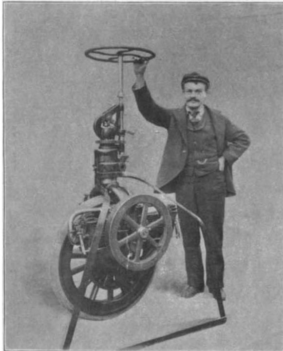
Fig. 1.—A DETACHED MOTOR-WHEEL, SHOWING THE MOTOR, FLY-WHEEL, AND STEERING GEAR.
