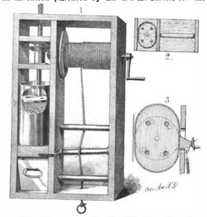
PERSPECTIVE AND SECTIONAL VIEWS OF THE FIRE-ESCAPE AND LOWERING APPARATUS.
