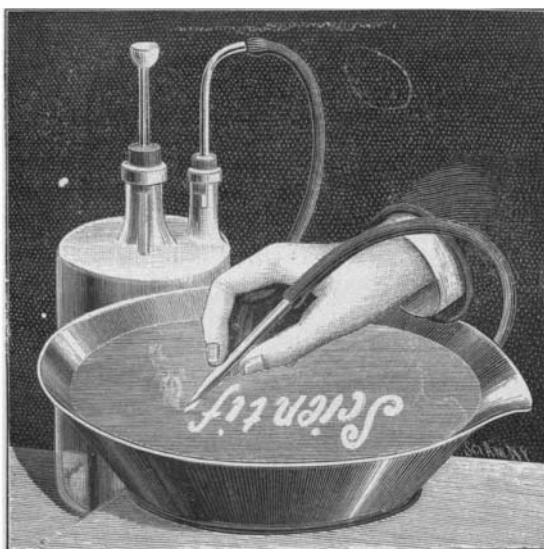
Fig. 3.—WRITING UPON WATER WITH HYDROSULPHURIC ACID.
