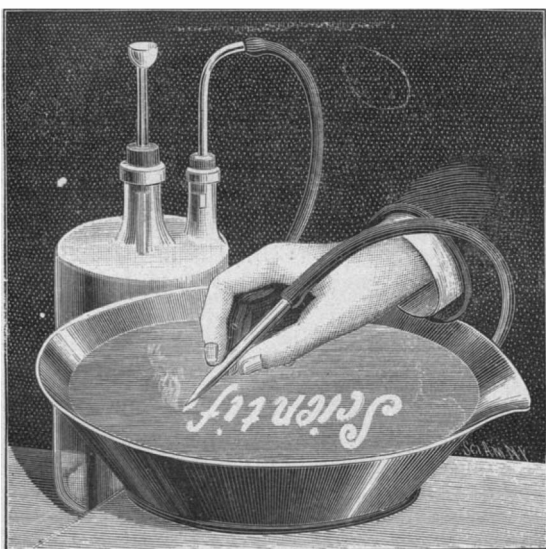
Fig. 3.—WRITING UPON WATER WITH HYDROSULPHURIC ACID.
