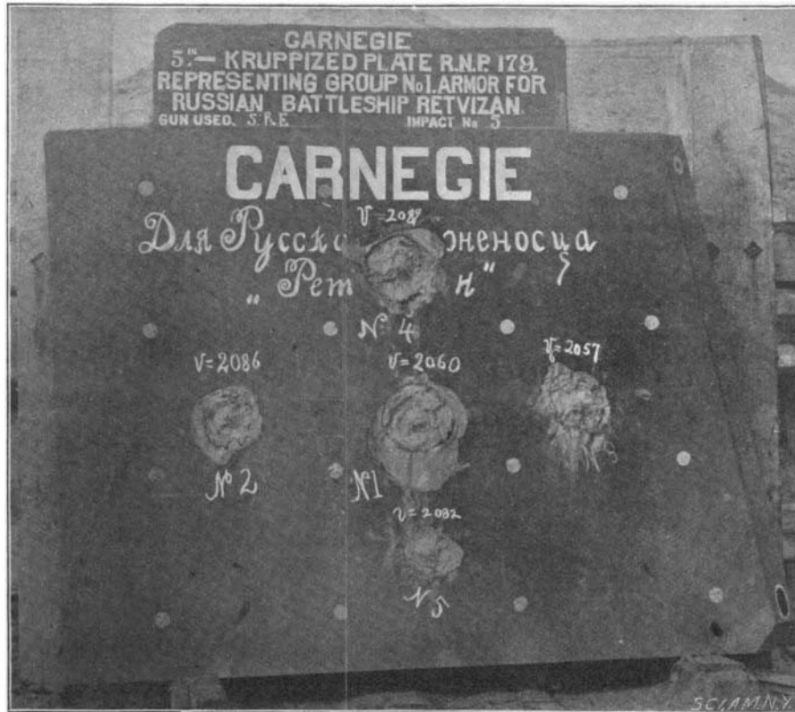
Fig. 1.—TEST OF 5-INCH KRUPP PLATE FOR RUSSIAN BATTLESHIP "RETVIZAN." Impact No. 5 by 5-inch, 50-pound projectile; striking velocity, 2,082 feet per second; striking energy, 1,502 tons. Projectile smashed, point welded to plate, penetration 2 inches. Penetration on similar Harveyized plate would have been 4.4 inches.
