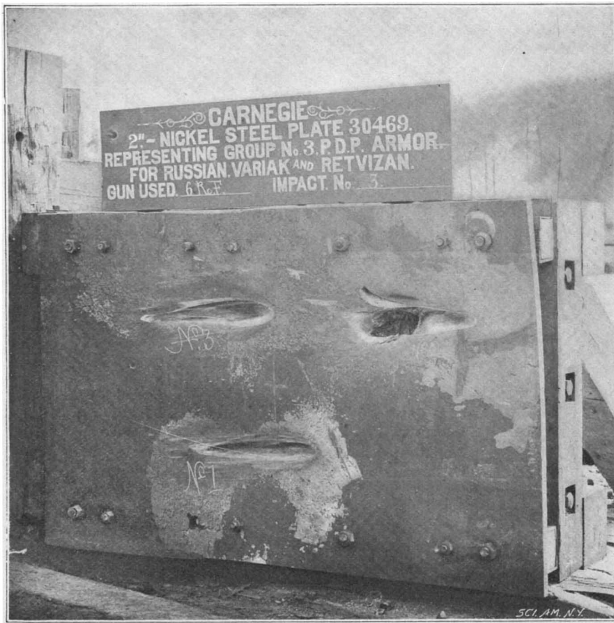
Fig. 2.—TEST OF 2-INCH NICKEL-STEEL PLATE.
