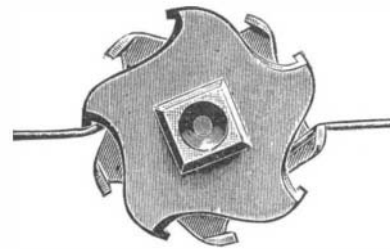
SIDE VIEW, SHOWING MANNER OF FASTENING THE WIRE.
