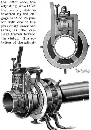
ing-shaft will cause the tool to be automatically fed toward the pipe in order to cut a taper thread. The tool may be fed away from the pipe by bringing the other rack into engagement with the pinion. When it is desired to cut a pipe, the carriage-sleeve is loosened so that it will not turn with the carriage; by this means the carriage will be held in one position relative to the pipe, and the cutting-tool may be fed inwardly by hand, until the pipe has been severed.
