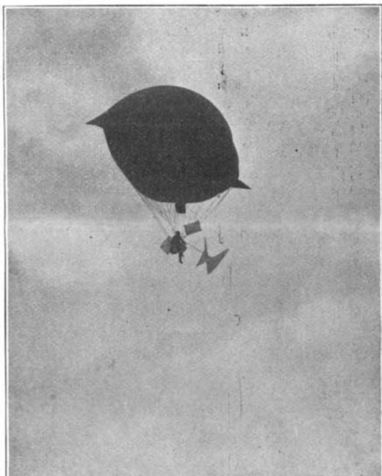
SPIRAL DESCENT OF THE "SKYCYCLE," SHOWING POSITION OF SCREW, SAIL, AND PLANES.
