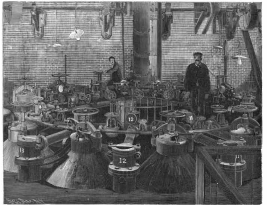
The Diffusion Cells, where the Sugar is Soaked Out.
