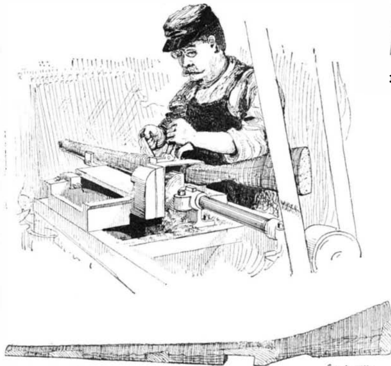
10.—Slotting the Stock—Roughing Cut Preparatory to Bedding.
