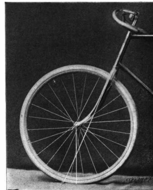
The Two White Cords show the Axis of the Head and the Point of Contact of the Wheel.
