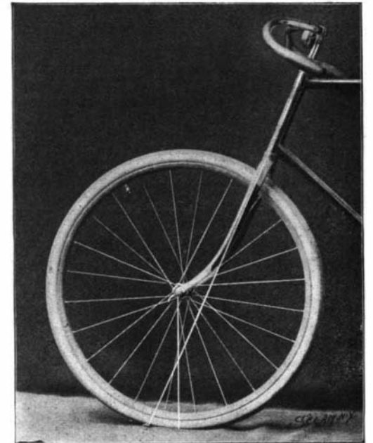
The Two White Cords show the Axis of the Head and the Point of Contact of the Wheel.
