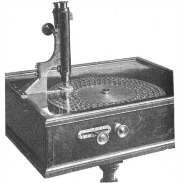
CLASS MICROSCOPE ARRANGED FOR EXAMINING FORAMINIFERA.
