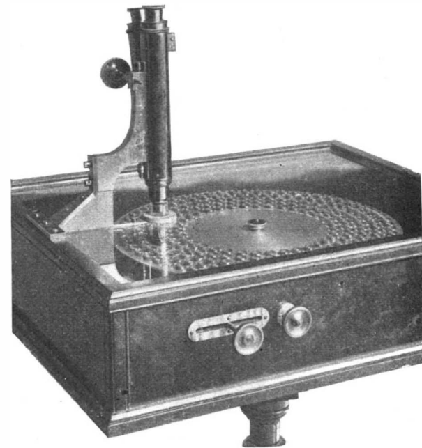
CLASS MICROSCOPE ARRANGED FOR EXAMINING FORAMINIFERA.
