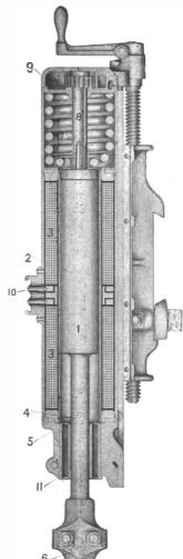
Fig. 2.—LONGITUDINAL SEC- country. This mine was TION OF THE MARVIN once famous for its nickROCK DRILL.
