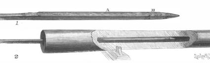
6.-Finish Reaming Bore of Barrel.
