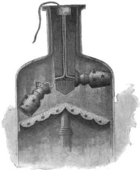
METHOD OF LOCKING THE STOPPER-ARMS.
