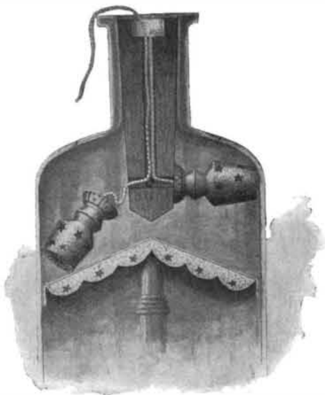
METHOD OF LOCKING THE STOPPER-ARMS.
