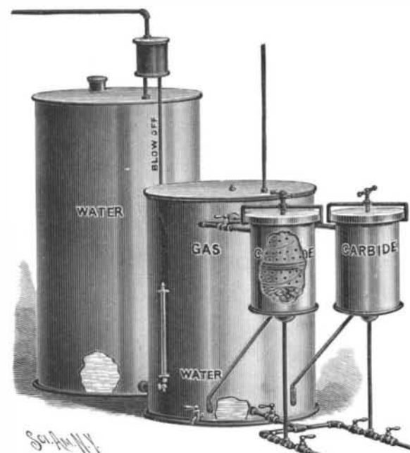
KEISER'S AUTOMATIC ACETYLENE-APPARATUS.
