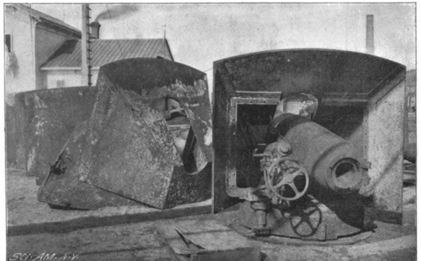
2.—VIEW SHOWING BREECH AND MOUNTING OF A 5 1/2-INCH GUN.
