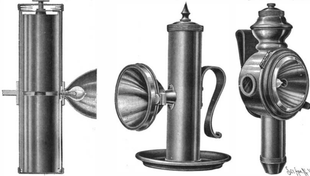
Fig. 1.—An Electric Bicycle-lamp in Partial Section.
