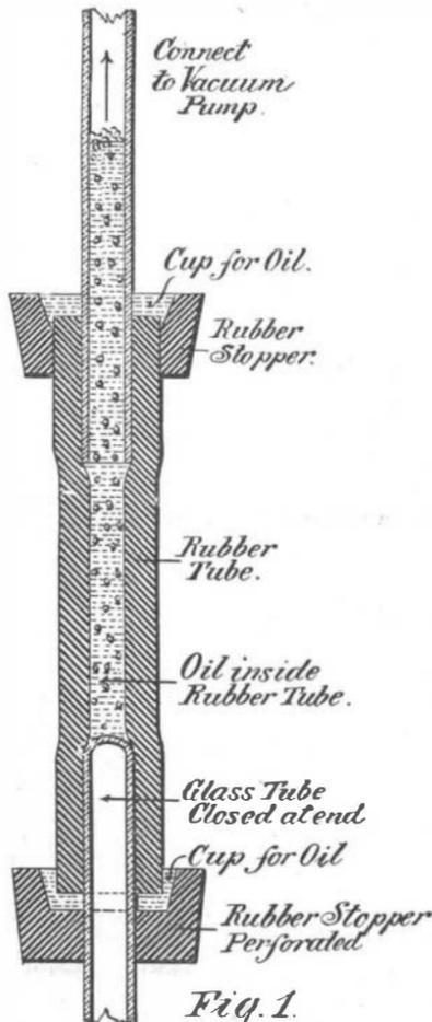
METHOD OF TESTING LEAKAGE IN BICYCLE TIRES.
