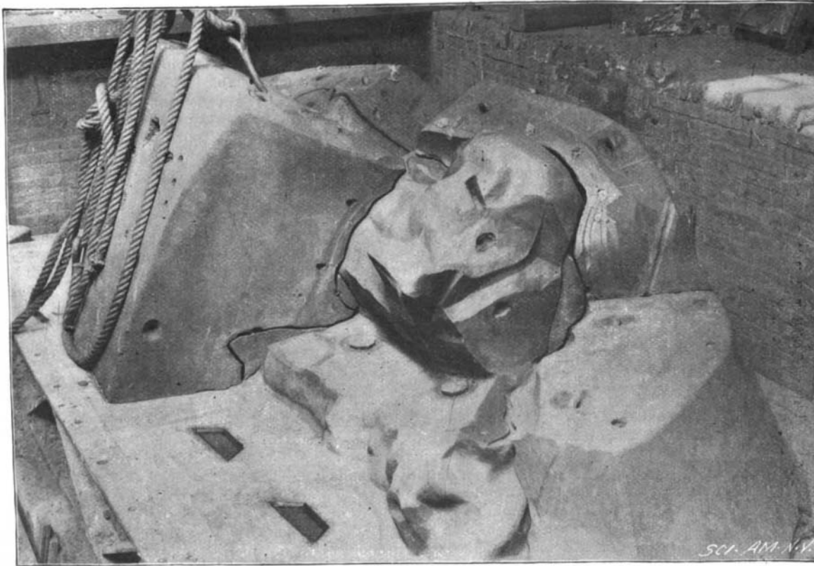
PART OF MOULD AND CORE SHOWING SPACE OCCUPIED BY THE METAL.
