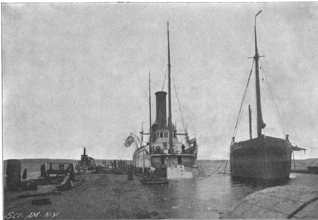
ACCIDENT TO THE "GRESHAM" AFTER BEING DIVIDED TO PASS THROUGH ST. LAWRENCE CANALS.
