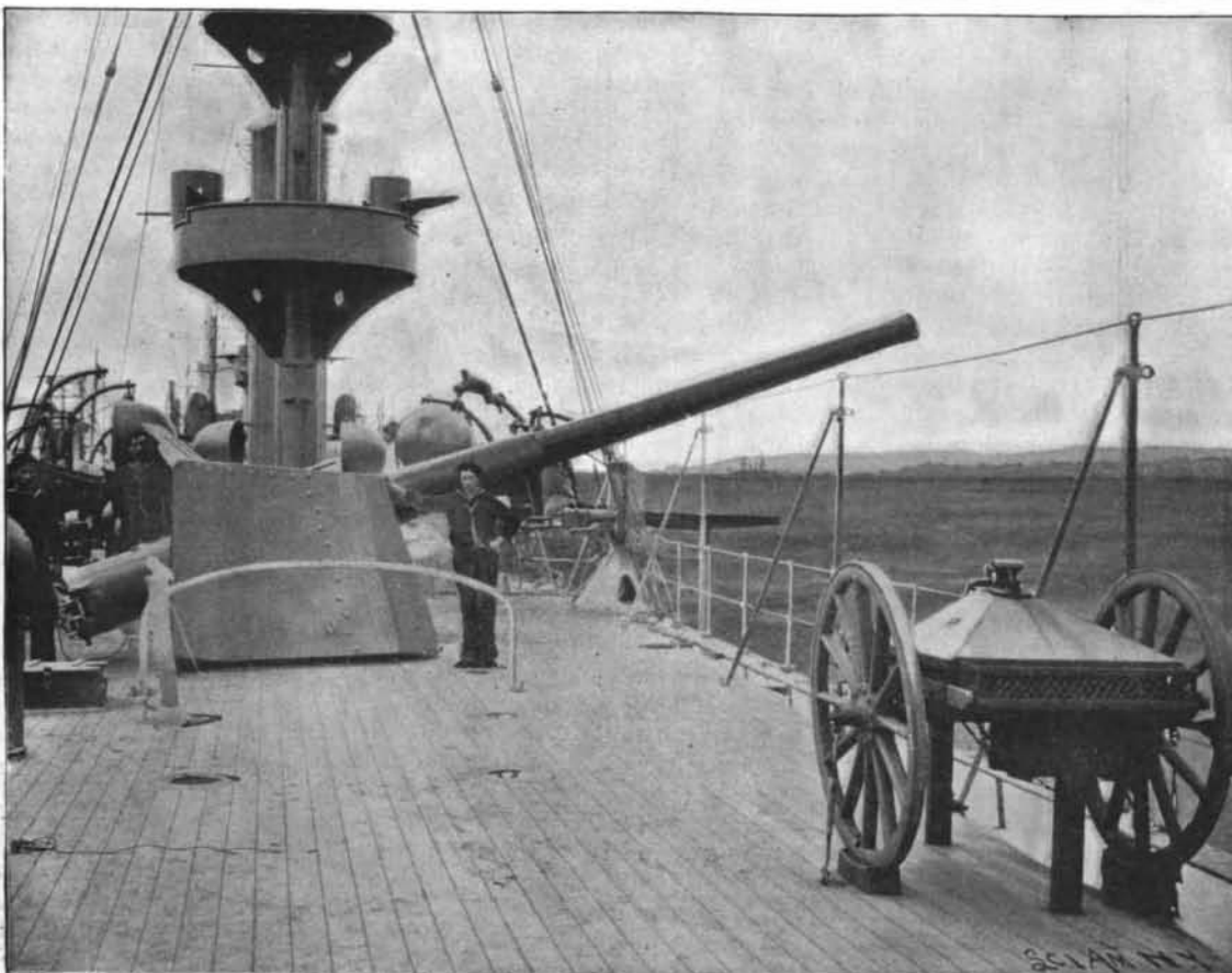
Fig. 2.—A 6-INCH RAPID-FIRE GUN ON THE "NEW ORLEANS" AT ITS MAXIMUM ELEVATION FOR RANGE OF SIX MILES.
