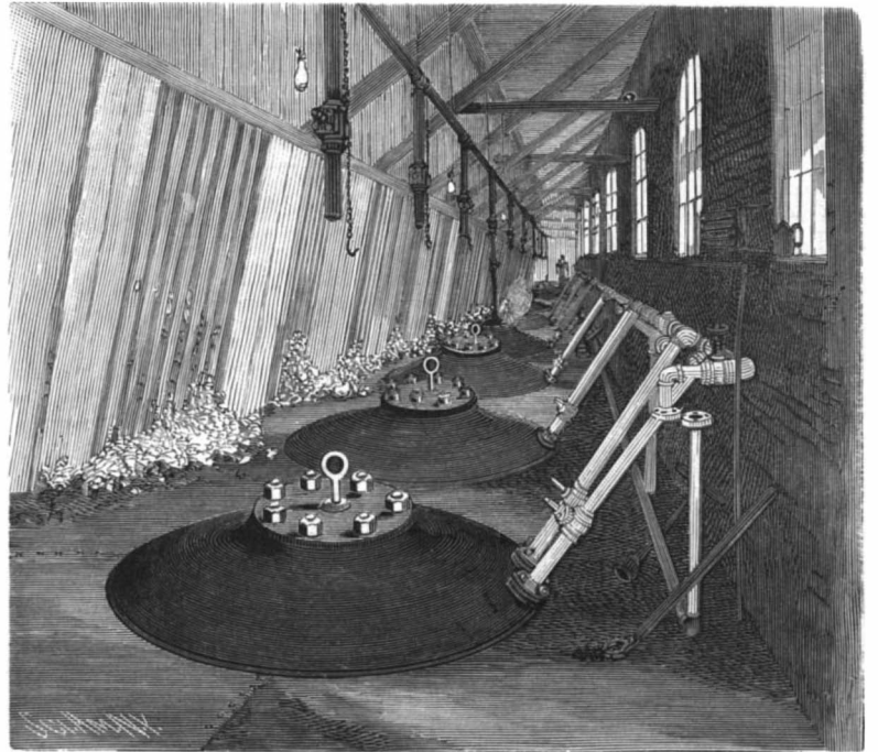
Fig. 1.—A BATTERY OF SODA DIGESTERS—VIEW ON CHARGING FLOOR, SHOWING BINS FOR CHIPS, THE MANHOLES, ETC.
