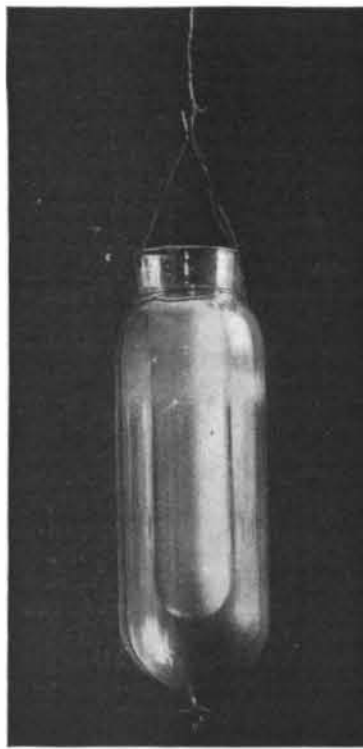
Fig. 2.—TUBE SURROUNDED BY CROOKES' VACUUM.
