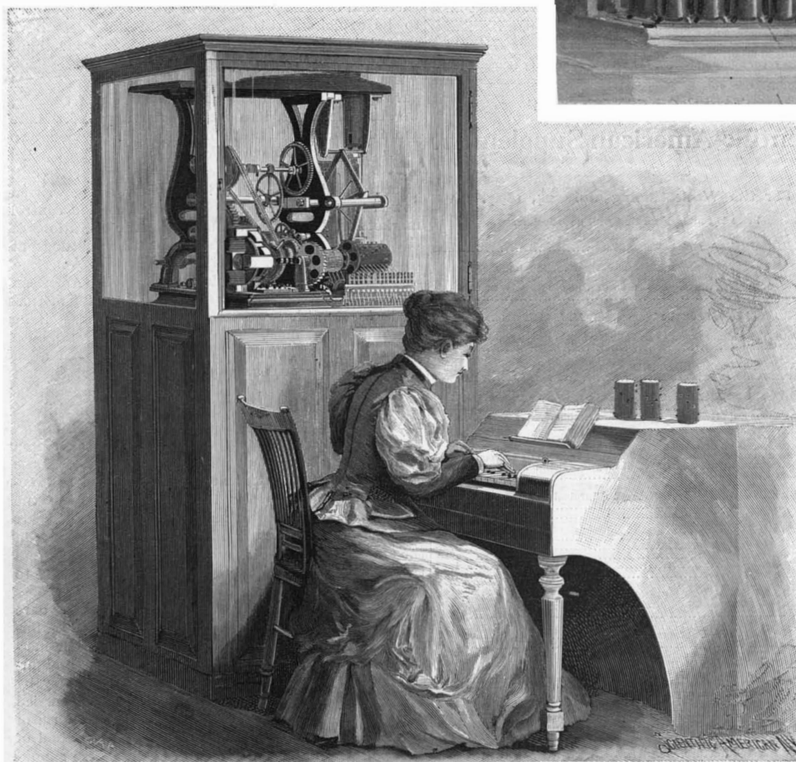
ELECTRIC SELF-WINDING CLOCK AND KEYBOARD. ELECTRIC TOWER CLOCK AND CHIMES, GRACE CHAPEL, NEW YORK.
