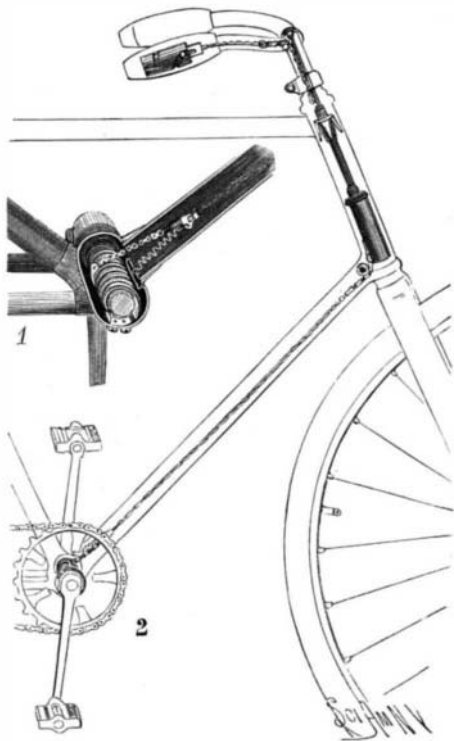
1. Detail view of coil. 2. Connections between coil and handle bar.
