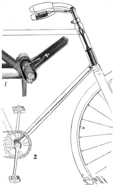
1. Detail view of coil. 2. Connections between coil and handle bar. THE SPENCER INVISIBLE COIL BRAKE.
