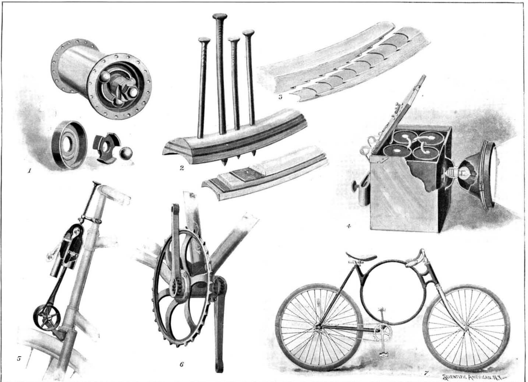
1. Three-ball bearing. 2. Non-splittable rim. 3. Joint for non-splittable rim. 4. Electric bicycle lamp. 5. Automatic whistle. 6. A device to reduce friction. 7. The circle cycle.
