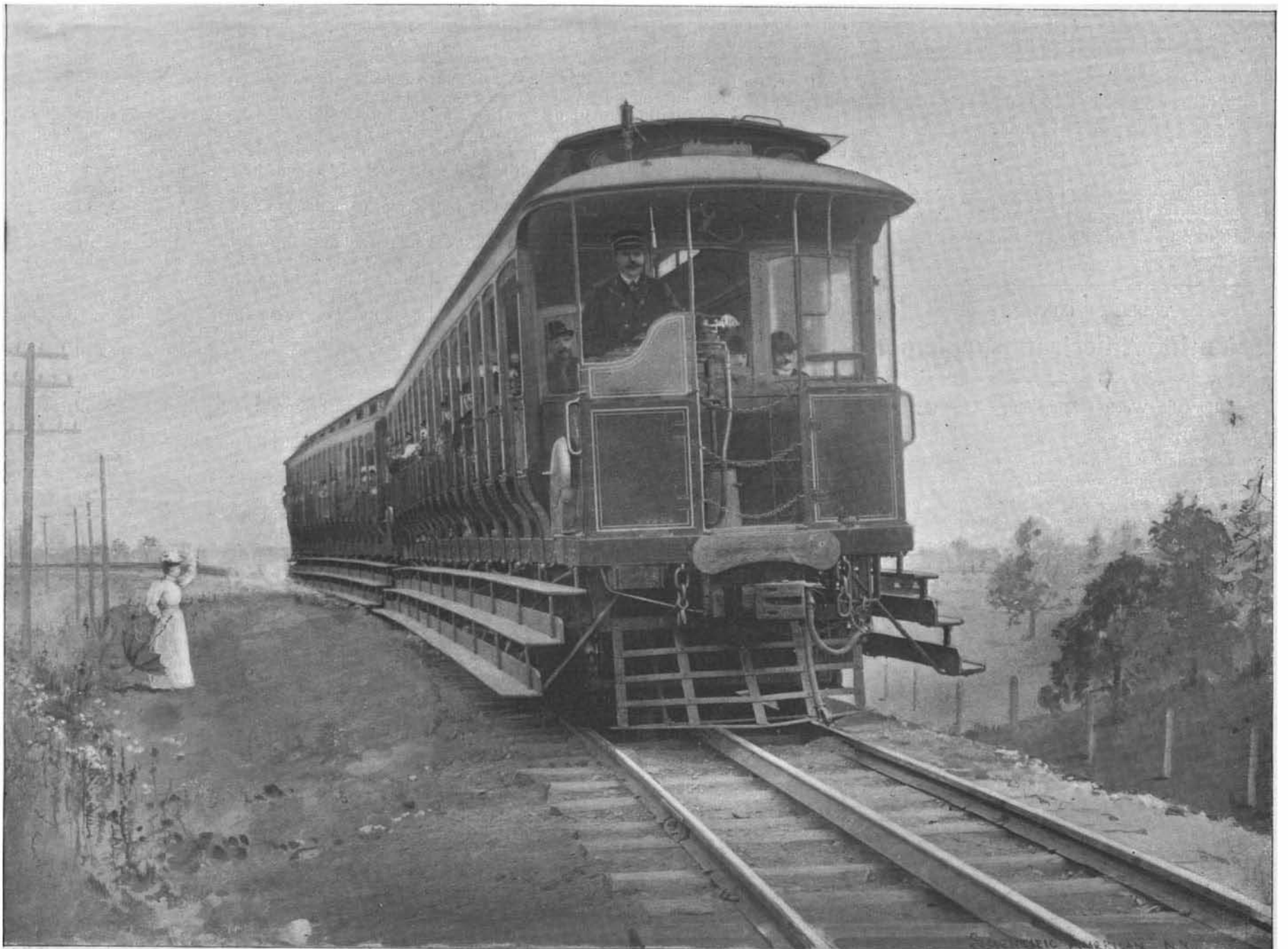
TRAIN CONSISTING OF A MOTOR CAR AND ONE COACH RUNNING AT FULL SPEED. THIRD RAIL ELECTRICAL EQUIPMENT OF THE NEW YORK, NEW HAVEN AND HARTFORD RAILROAD.—[See page 376.]
