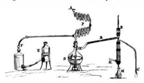
APPARATUS FOR MAKING ALCOHOL BY MEANS OF ACETYLENE GAS.
