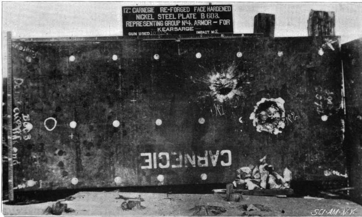
TEST OF FACE-HARDENED NICKEL STEEL SIDE ARMOR FOR THE KEARSARGE.
