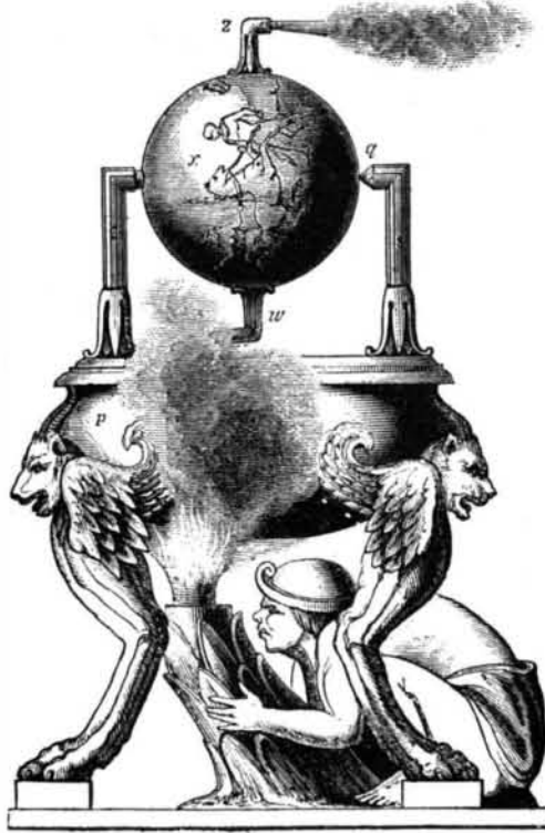
THE GRECIAN IDEA OF HERO'S STEAM ENGINE. 120 B. C.
