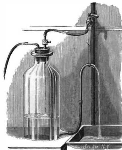
Fig. 2.—ASPIRATOR ARRANGED FOR PRODUCING A BLAST.
