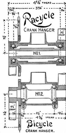
Cut No. 1 is a sectional view of the RACYCLE Crank Hanger.
