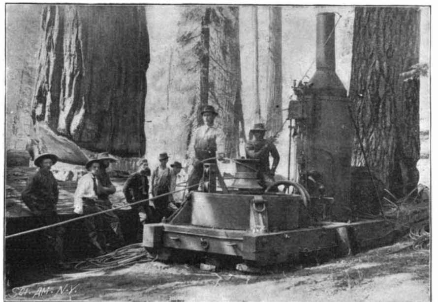
LOGGING IN THE SIERRA NEVADAS—PORTABLE DONKEY ENGINE HAULING LOGS.
