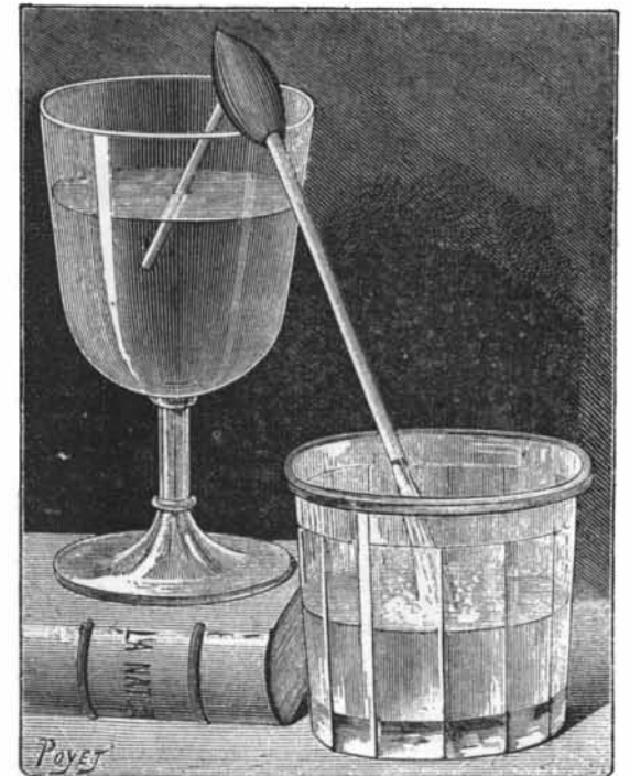
SIPHON MADE OF A STRAW AND A PEACH PIT.
