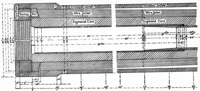
LONGITUDINAL AND CROSS SECTIONS SHOWING CONSTRUCTION OF THE TEN INCH BROWN SEGMENTAL WIRE GUN.
