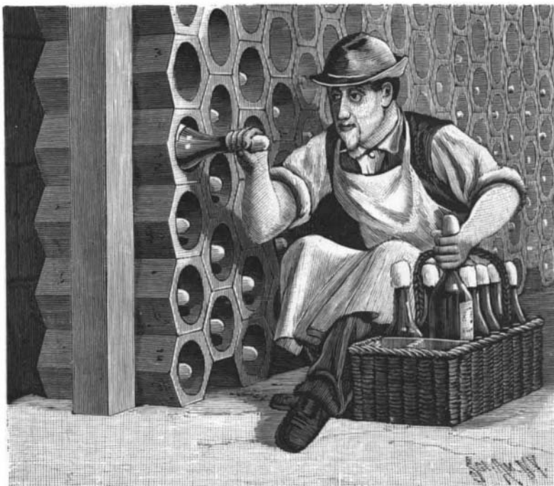
HONEYCOMB WINE BINS OF VITRIFIED CLAY PIPE.
