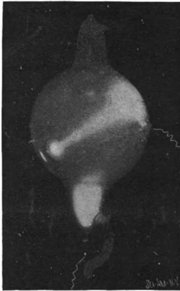
Fig. 1.—CATHODE BEAM IN CROOKES TUBE, DIAGONAL VIEW.
