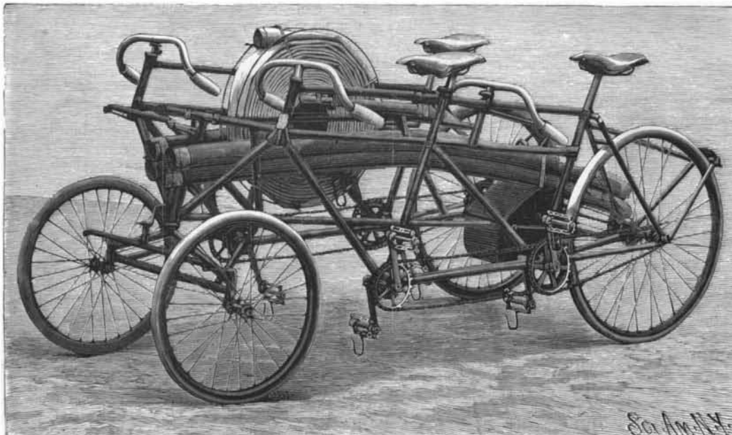
Fig. 1.—THE SCHOEDELIN QUADRICYCLE FIRE ENGINE.
