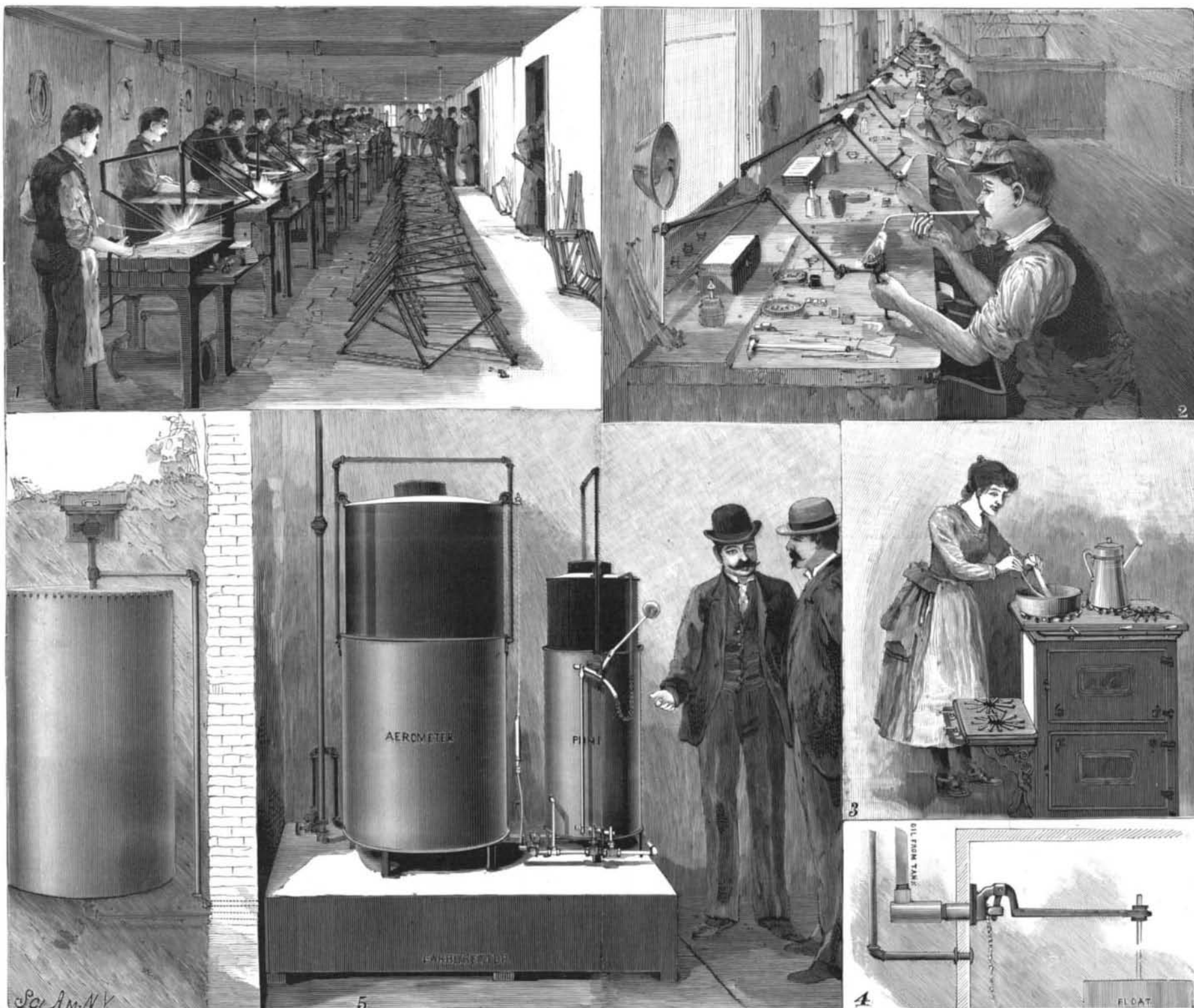
1. Brazing bicycle frames. 2. Making jewelry. 3. The gas stove at home. 4. The automatic gasoline valve. 5. The complete gas apparatus.
