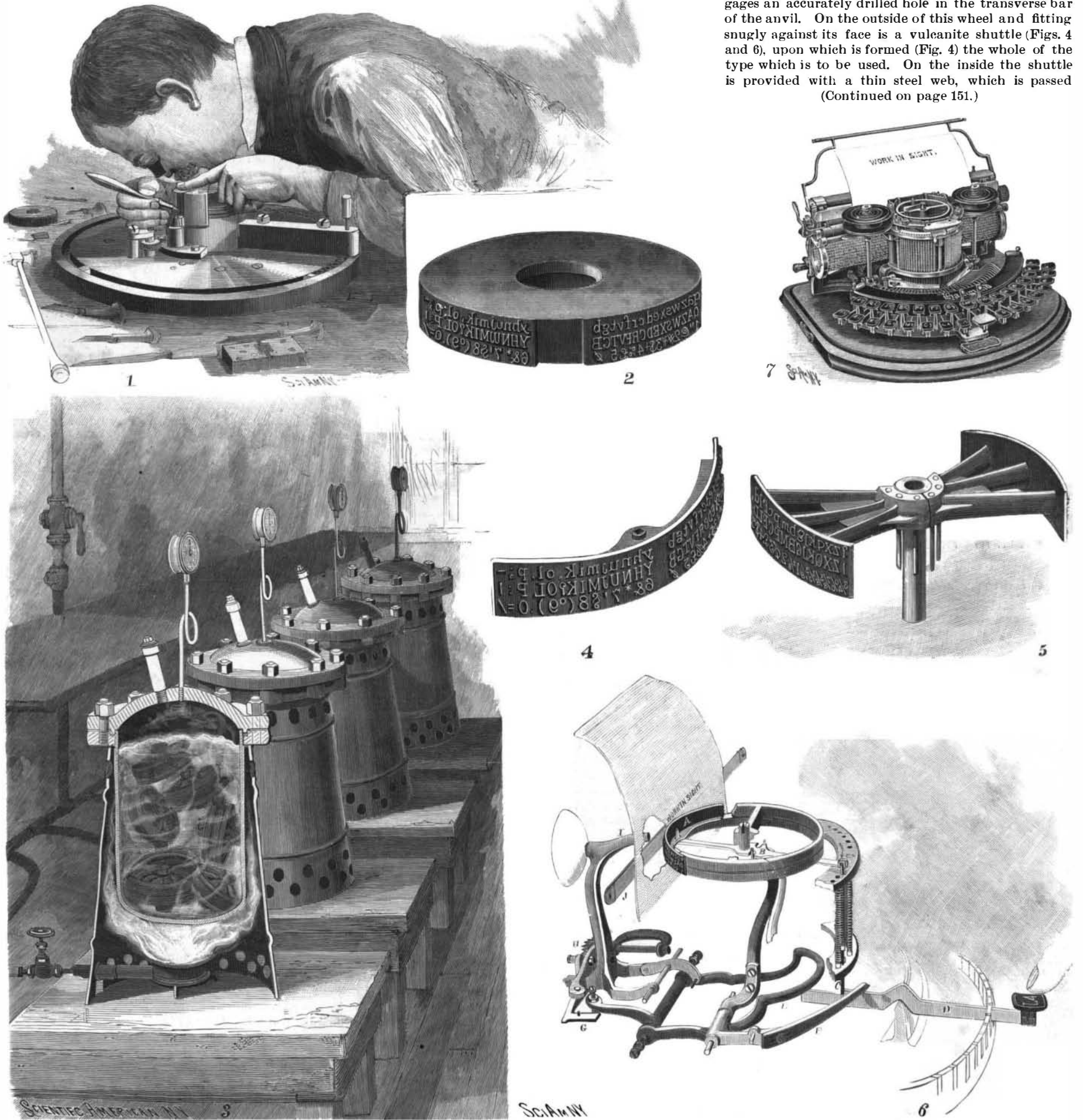
1. Marking the location of the type. 2. Steel wheel, with type engraved. 3. Vulcanizing plant. 4. Vulcanite shuttle, showing steel web. 5. Original form of shuttle, in two parts. 6. Detail view of type bar and hammer mechanism. 7. The Hammond typewriter complete.
