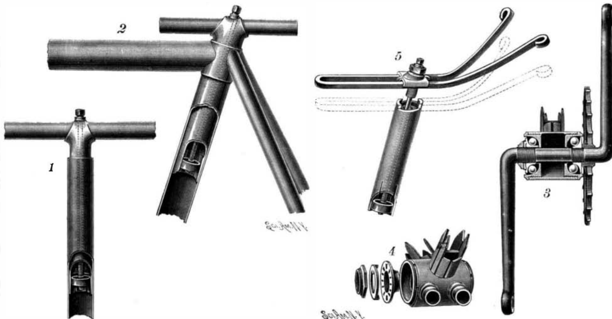
BICYCLE FRAME IMPROVEMENTS—HANDLE BAR, SEAT POST, CRANK AND SADDLE CONNECTIONS.
