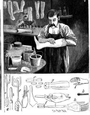
5. Carving leg sections by hand. 6. Details and parts of artificial limb making.
