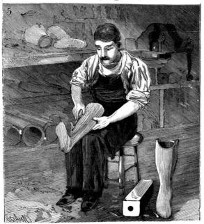
tion was constructed by Mr. A. A. Marks during the interim 1853-1863. The joint included a spring adjustable for tension and provided compensation for wear. The experience of ten years showed that the ingenious and much praised ankle joint was too weak for hard service, and repairs were
