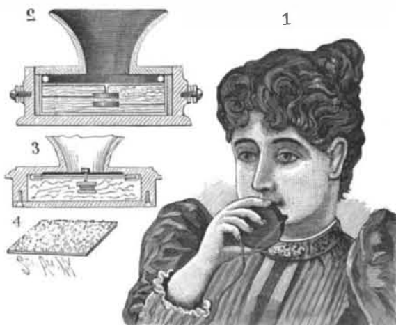
LUCAS' TELEPHONE TRANSMITTER.
