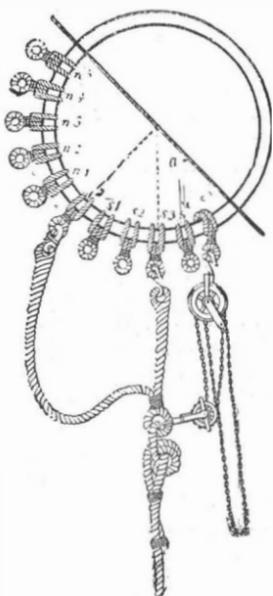
Fig. 3.—GUIDE ROPE ATTACHMENT.
