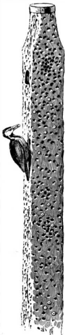
TELEGRAPH POLE BORED BY THE WOODPECKER.
